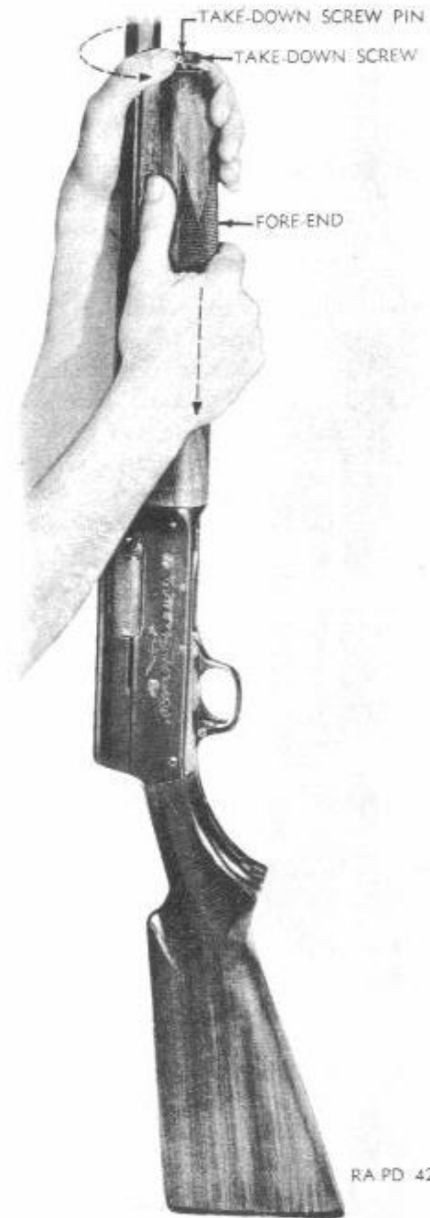
Figure 110—Disengaging Take-down Screw While Holding Fore End Against Spring Tension—Remington Shotgun, Sportsman
